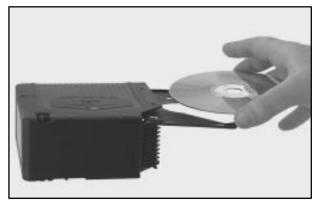
You must first load the magazine with discs before you can play a compact disc. Each of the 12 trays holds one disc. Load the trays from top to bottom, placing a disc on the tray label side up. If you load a disc label side down, the disc will not play and an error will occur. Gently push the tray back into the magazine slot until it locks into place. Repeat this procedure for loading up to 12 discs in the magazine.
