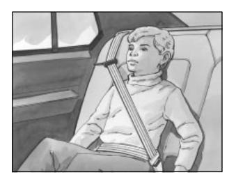
Buckle, position and release the safety belt as described in "Rear Seat Passenger Positions" earlier in this section. Make sure that the shoulder belt crosses the shoulder. To remove and store the comfort guides, squeeze the belt edges together so that you can take them out from the guides. Slide the guide into its storage pocket on the side of the seatback.
