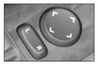
The controls on the driver's door operate both outside rearview mirrors. Move the L/R switch to the left (L) to select the driver's side rearview mirror, or to the right (R) to select the passenger's side rearview mirror.
