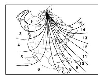
3. Once the zone number appears in the display, press the COMPASS (or the on/off button for mirrors equipped with OnStar controls) button quickly until the correct zone number appears in the display. Stop pressing the button and the mirror will return to normal operation. If "C" appears in the compass window, the compass may need calibration. See "Compass Calibration" explained previously.
