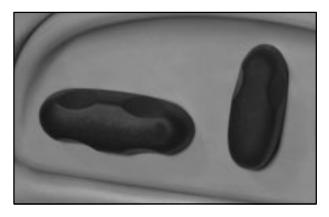
The power seat controls are located on the outboard side of each front seat.
