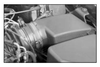
The engine air cleaner and filter are on the driver's side of the engine compartment. See "Engine Compartment Overview" in the Index for more information on location. To check or replace the air filter:
