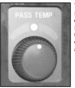
With this feature, the right front seat passenger can control the comfort setting for their own zone. To use this feature, turn the knob on the passenger's door to a cooler or warmer setting.
