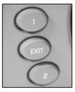
If your vehicle has this feature, the controls on the driver's door panel are used to program and recall previous settings.
