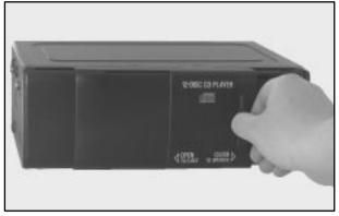
Once you have loaded the discs in the magazine, slide open the door of the compact disc (CD) changer. Push the magazine into the changer in the direction of the arrow marked on top of the magazine. Close the door by sliding it all the way to the right. When the door is closed, the changer will begin checking for discs in the magazine. This will continue for up to one and a half minutes depending on the number of discs loaded.
