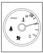
This gage shows the engine coolant temperature. If the gage pointer moves into the red warning zone, your engine is hot.
