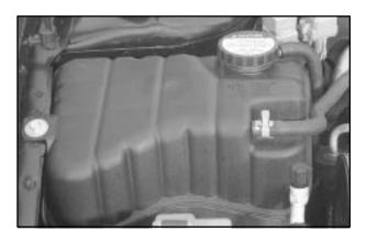
The engine coolant surge tank is located on the passenger's side of the engine compartment. See "Engine Compartment Overview" in the Index for more information on location.
