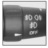
To turn on only the front fog lamps, turn the fog lamp band to the single fog lamp symbol. To turn on both the front and rear fog lamps, turn the fog lamp band to the double fog lamp symbol.
