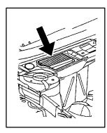
The passenger compartment air filter is located on the passenger side at the base of the windshield and can be accessed through a removable panel under the hood of the vehicle.
