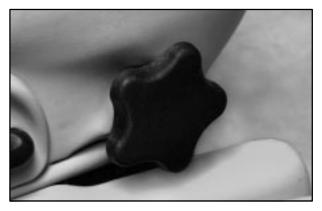
The knob that controls this feature is located on the outboard side edge of the seat. Turn the knob towards the front of the vehicle to increase lumbar support. Turn the knob towards the rear of the vehicle to decrease lumbar support.
