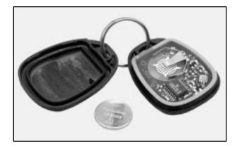
For battery replacement, use a Duracell  $^{\circledR}$  battery, type DL-2032, or a similar type.
