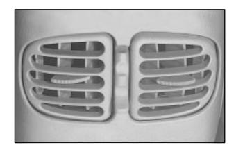
Turn the control between the rear outlets up to direct air through the upper outlets. Turn the control down to direct air through the lower outlets. Adjust the direction of airflow from side to side with the controls in each outlet.
