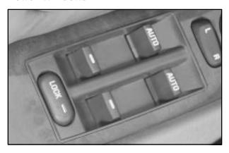
Switches on the driver's door armrest control each of the windows while the ignition is on or retained accessory power (RAP) is active. In addition, each passenger's door armrest has a window switch for its own window.
