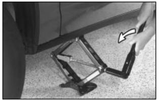
3. Turn the wheel wrench counterclockwise by hand to lower the jack head until it fits under the vehicle.
