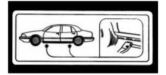
4. Near each wheel well is a notch in the frame to position the jack head. Position the jack under the vehicle and raise the jack head until it fits firmly against the sheet metal. Do not raise the vehicle yet. Put the compact spare near you.
