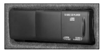
With the optional compact disc changer, you can play up to 12 discs continuously. Normal size discs may be played using the trays supplied in the magazine.
