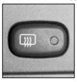
REAR: Press this button to warm the defogger grid on the rear window. An indicator light below the button will glow while the rear window defogger is operating.
