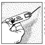
To do so, first open the trunk. The release mechanism is located on the driver's side of the vehicle, at the top of the trunk compartment. Pull the tab toward you to release the fuel door.
