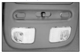
These lamps and the interior courtesy lamps will come on when you open a door. They will turn off when you turn on the ignition. If a door is left open, they will turn off after about 10 minutes.
