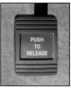
Your vehicle has a PUSH TO RELEASE parking brake. To set the parking brake, hold the regular brake pedal down with your right foot. Push down the parking brake pedal with your left foot.
