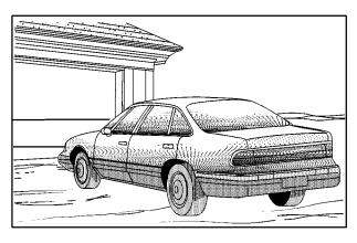
4. Turn on the low beam headlamps and cover the lamp not being evaluated. The ambient light should allow the beam cut off to be seen on the wall.
