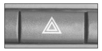
To turn on the hazard warning flashers, press and release the button located in the center of the instrument panel. The indicators for the turn signals will flash on and off.
