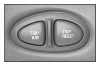
Press the TRIP A/B button to change which trip odometer is displayed.
