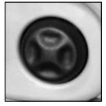
The power lumbar controls are located on the outboard side of each front seat.
