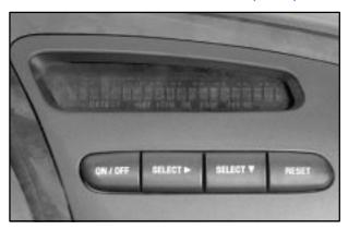
The Driver Information Center (DIC) displays information in either English or metric. When the system is on or off, push the ON/OFF button down for three seconds to change the display between English and metric. This will also change the digital screen for the climate control system between English and metric.
