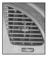
The direction of the air can be controlled by adjusting or closing the outlets in the instrument panel.
