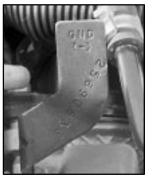
If you have the 4.0L V8 engine, your vehicle has a remote negative terminal, marked "GND", located near the power steering fluid reservoir. Attach the cable to the remote negative terminal provided.
