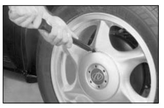
Insert the hooked end of the wheel wrench in one of the two small notches in the center cover and pry the cover off. Do not drop the cover or lay it face down, as it could be scratched or damaged.
