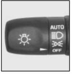
The headlamp control is located on the turn signal/multifunction lever.
